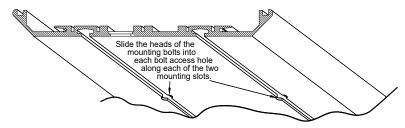
4. Slide two bolts in each channel, one towards each end. You will use two bolts on each end (one in each channel) to secure the mounting bracket.
